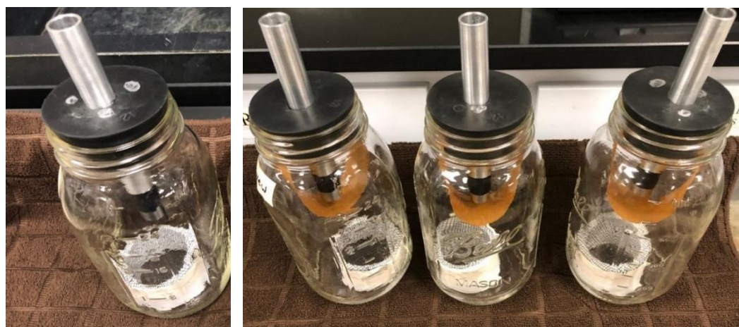
Figure 1: VIA test setup for VCI impregnated wrapper corrosion effectiveness evaluation.
