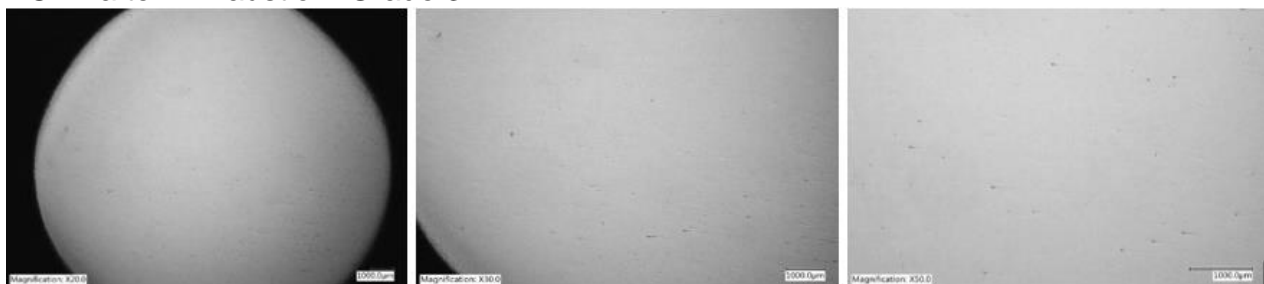
VCI E + super hydrophobic after Exhaustion VIA test, Grade 4.
